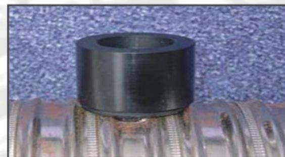
Grouting Port in Steel Sheath
